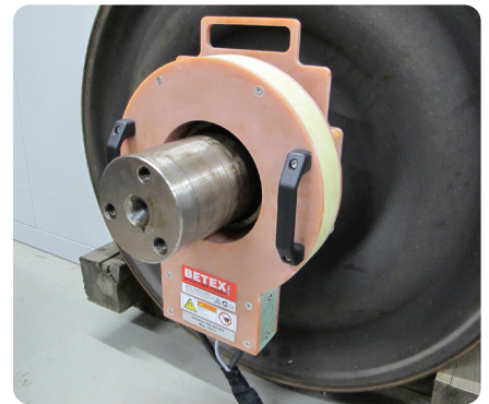
Heating labyrinth rings for dismounting
