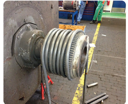
Heating a coupling for dismounting
